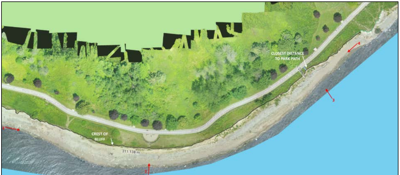
Figure 30. 3D model of RPAS photogrammetry data used to create a plan view of the deficiencies and photo locations for Site E (EMS983). Source: TRCA, 2021.
