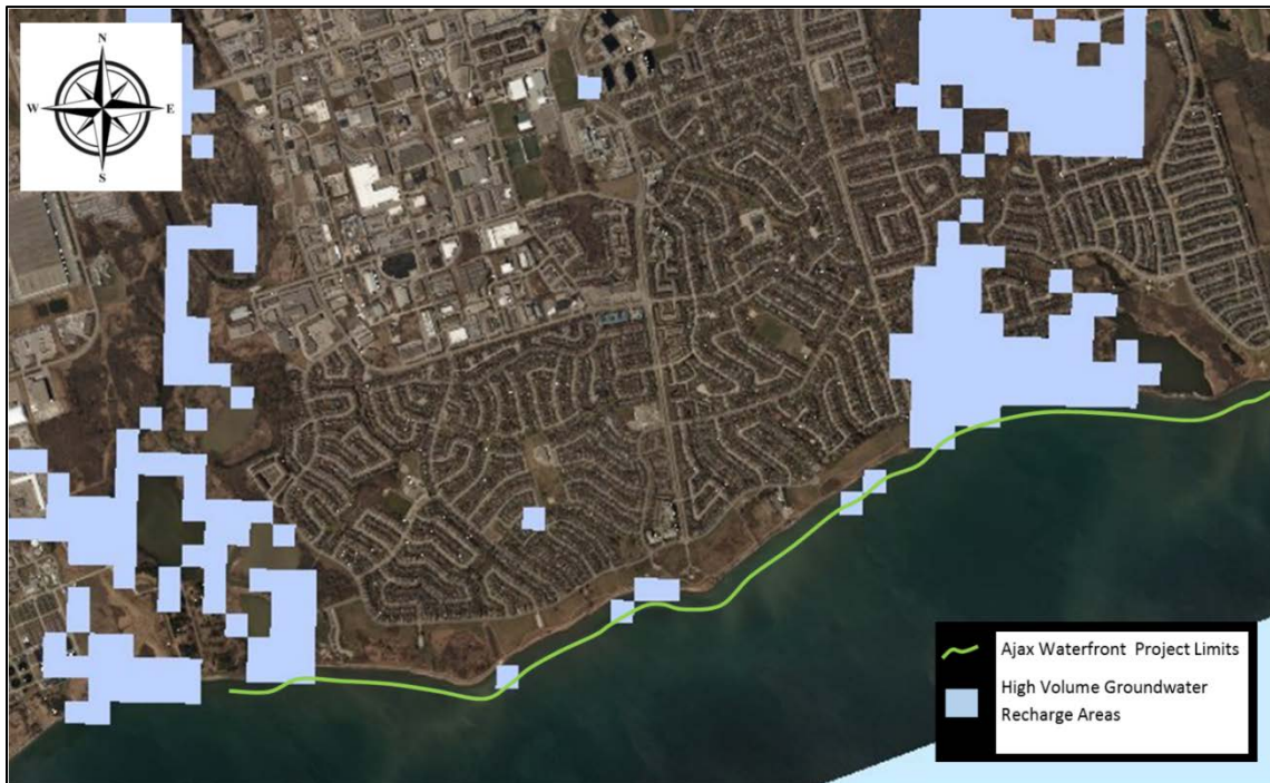
Figure 13. Groundwater recharge areas near and within the project area. Source: TRCA, 2021.
